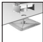
Recessed Mounting via round hole
