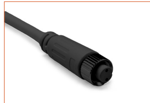
FCB-2P-67 Female connector, 30cm (0.98ft) black cable, 2 pin, IP67, Wet, 20 AWG
