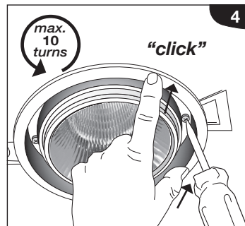
4. Repeat Step 2 by unscrewing second beam direction locking screw.*
