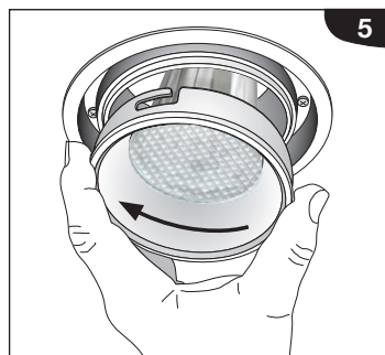
5. Re-assemble Reflector Assembly (Reflector, IP54 Lens and thermoplastic Ring) and install assembly into downlight by turning clockwise.
