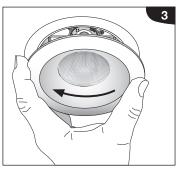
3. Re-assemble Reflector Assembly (Reflector, Lens and Ceiling Ring) and install assembly into downlight by turning clockwise. Ensure reflector is fully seated into ceiling ring.
