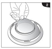
2. Recessed Reflector Option - fit Lens Accessory into Ceiling
