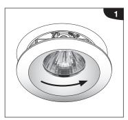
1. Remove ceiling ring/reflector assembly (turn anti-clockwise).
