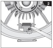
2. Disengage tail of torsion spring by pushing tail behind lug.
