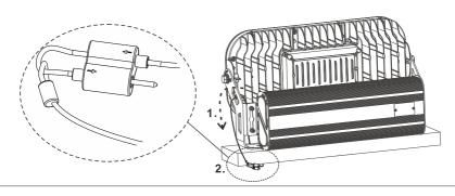
\* Please select the appropriate power cord according to the total power of interconnected lamps.
