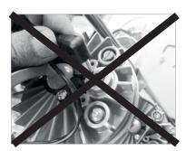
1.3 - to turn the KIDLED module, undo the screw with a 3-mm Allen key
