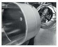
2.3 - Unplug the KIDLED modules. Checking that the polarity is correct
