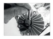
2 - FIXATION ON THE POLE 2.1 - Undo the 3 screws with a 4-mm
