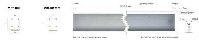
Fixture build to length (not field cutable): L = (N x 62.5 mm) + 21 mm; N = 1 ... (as follows); L<sub>min</sub> = 84 mm; HD6/HD10/HD15: Nmax = 64; L<sub>max</sub> = 4,021 mm; HD25: Nmax = 48; L<sub>max</sub> = 3,021 mm
